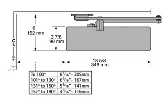
Butt Hinges should not exceed 5" (127mm) in width.
