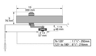
To 120° 5<sup>7</sup>/<sub>8</sub>" - 149mm 121° to 180° 3<sup>11</sup>/<sub>16</sub>" - 94mm 12 3/4 324 mm
